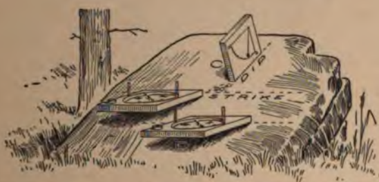
FIG. 28. — Diagram to illustrate the manner of determining the strike of rock beds at an outcropping. a, a compass which has the cardinal directions in their natural positions; b, a compass with the east and west initials reversed upon the dial; c, home-made clinometer in position to determine the dip.
